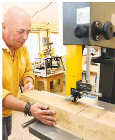
▲ Cutting this wet oak caused the saw to slow as it clogged in the cut
